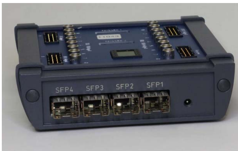
View of EXPLODER2C (SFP and auxiliary power supply side).
