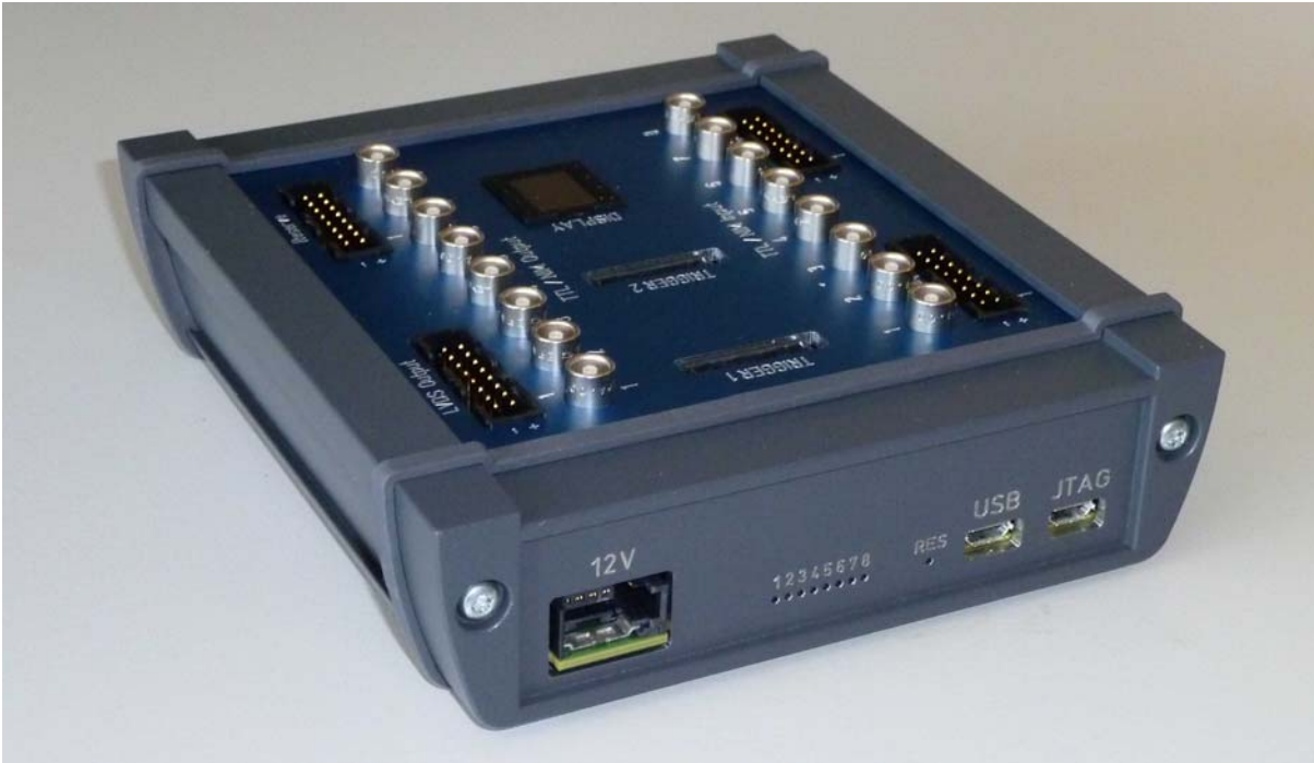
View of EXPLODER2C, (power supply side).
