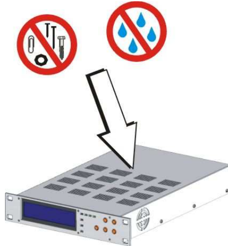
Fig. 1-2 Do not insert objects through louvers and keep device dry
