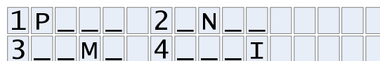
Figure 10 – display example, ch.1: active positive limit, ch.2: active negative limit, ch.3: active middle switch, ch.4: active interlock input
