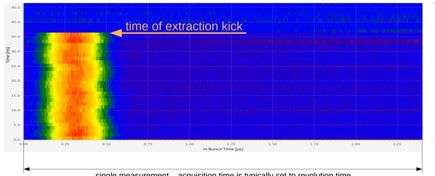
single measurement – acquisition time is typically set to revolution time start trigger: signal from DDS
