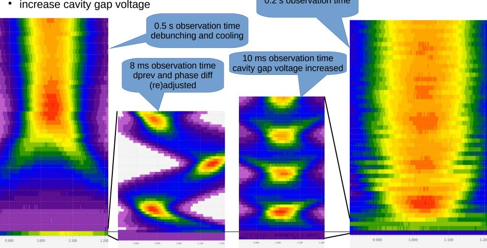
CRYRING extraction: the CRYRING team managed this without any help below: images of six consecutive extractions – the beam is always well centered
